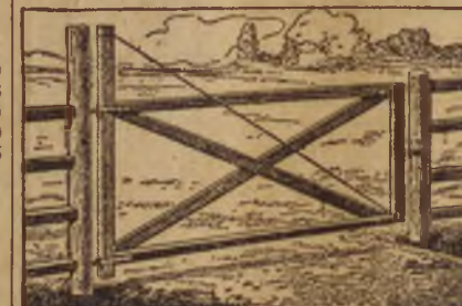
A Farm Gate That Will Not Sag Is Supported by a Diagonal Wire Brace.
