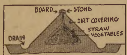
Cross Section of Storage Pit Containing Irish Potatoes During Severely Cold Weather the Dirt Covering May Be Supplemented by Manure, Straw, Etc.
