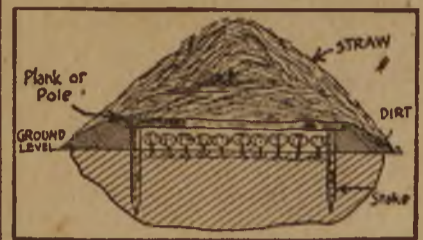
Fig. 1.—Cross Section of a Cabbage Storage Pit Made of Stakes and Poles and Covered With Straw—This Is a Good Way to Store Cabbages.
