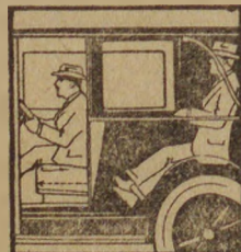
Front and rear seats adjustable forward and backward for tall and short people.
