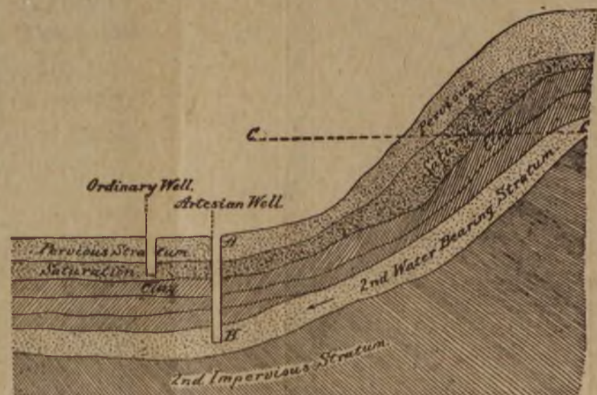
Geological Formation Showing Manner in Which Water Is Secured from Wells of Varying Depths.
