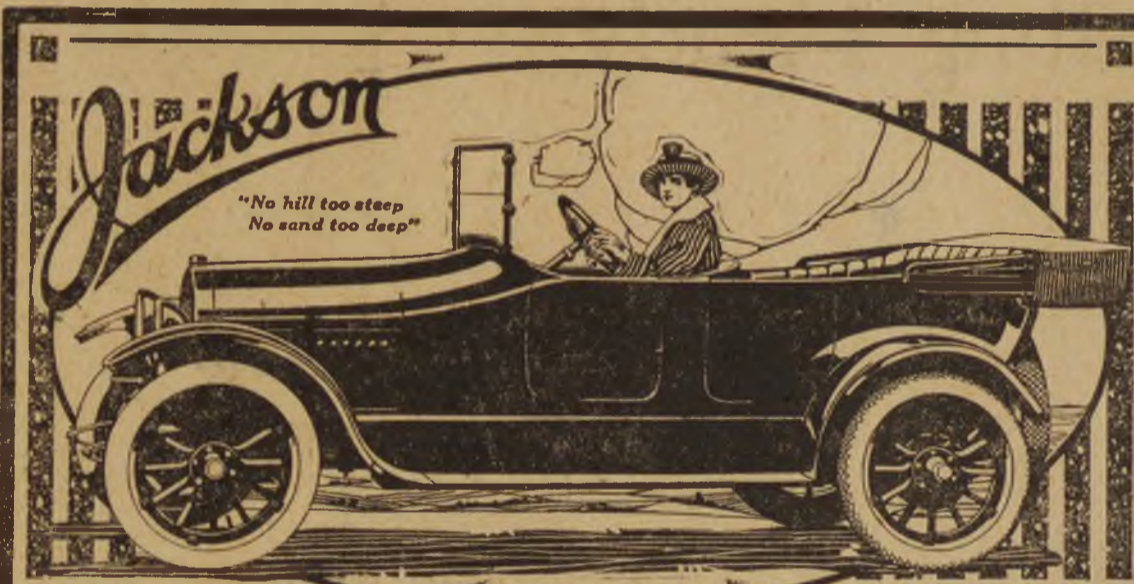
New Jackson Model "34"—motor 3 1/2 x 5"; 112-inch wheelbase; 32 x 4" tires—fully equipped, including one-man top, electric lighting and starting system, and Stewart Vacuum Fuel System
