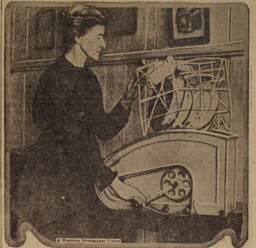
This machine which can be called the "Mechanical Maid," was invented in England to assist housewives in overcoming the servant shortage. Dishes sufficient for a three-course service for five persons can be washed up in this machine in a few moments. Photo shows dishes being put into machine.
