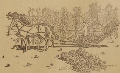
has the greatest success from the fact that it cuts and binds in the vertical position the only practical way to handle big corn that grows in fertile spots in every field, also because of our "locked joint" conveyor chain, the only chain ever made that will handle the stiff and stubborn corn stalks.
