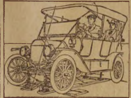
Car's Motor Does Work of Jacking.
