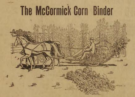
has the greatest success from the fact that it cuts and binds in the vertical position the only practical way to handle big corn that grows in fertile spots in every field, also because of our "locked joint" conveyor chain, the only chain ever made that will handle the stiff and stubborn corn stalks.
