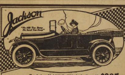
New Jackson Model "34"—112 inch wheelbase; 32 x4' tires—fully equipped, including one-man top, electric lighting and starting system, and Stewart Vacuum Fuel System.
