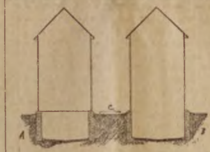
A. Incorrect Method of Constructing Silo Foundation. B. Correct Method. C. Ground Line.
